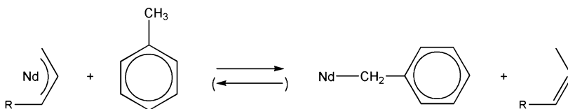
Scheme 13 Transfer of a benzyl-H-atom from toluene (solvent) to the allyl-end of a poly(butadien)yl chain [ R = \text{poly(butadien)yl} ] (ligands and charges are omitted for clarity) [422], reproduced by permission of Taylor & Francis Group, LLC., http://www.taylorandfrancis.com
